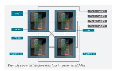
Infinity Fabric links, while four can be flexibly assigned to deliver either Infinity Fabric or PCIe Gen 5 connectivity.
